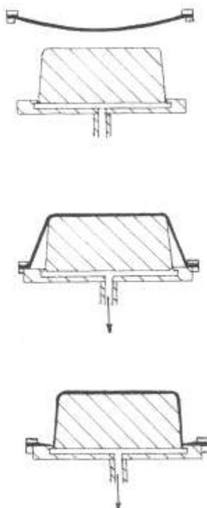
As with cavity forming, the last area to form is the thinnest. This avoids thin corners at the bottom as occurs with Cavity Forming, but is thinner at the rim (figure 3) and prone to forming webs. Cooling shrinkage can impede part removal.
